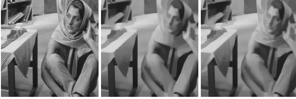
FIG. 6.2. Result of the algorithm on a natural image. From left to right: original image, Darbon-Sigelle's algorithm [27] using 4-connectivity, and average between two alternating sequential filters (one starting with opening the other with a closing, with squares as structuring element). Both images are very similar. Notice however that some details, for instance on the trousers, look different.
