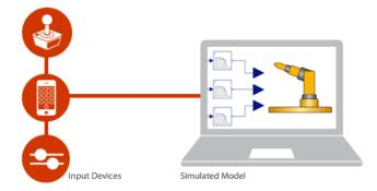
The ModelPlug library allows rapid prototyping of controllers without the need of writing a single line of code, thereby enabling interaction with complex simulation models and easy creation of realistic test scenarios.
