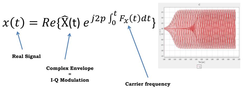
Scerne Allows to combine and handle <u>explicitly</u>  $x(t), \hat{X}(t)$  and Fx(t) within the same simulation, which offers flexibility and efficiency analysis
