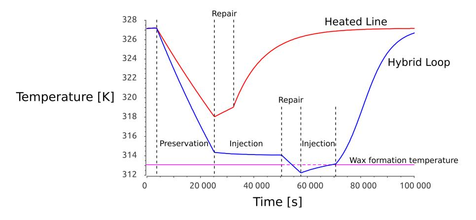
Fluid temperature comparison in the line at the sea bottom (active heating and hybrid loop architectures)
