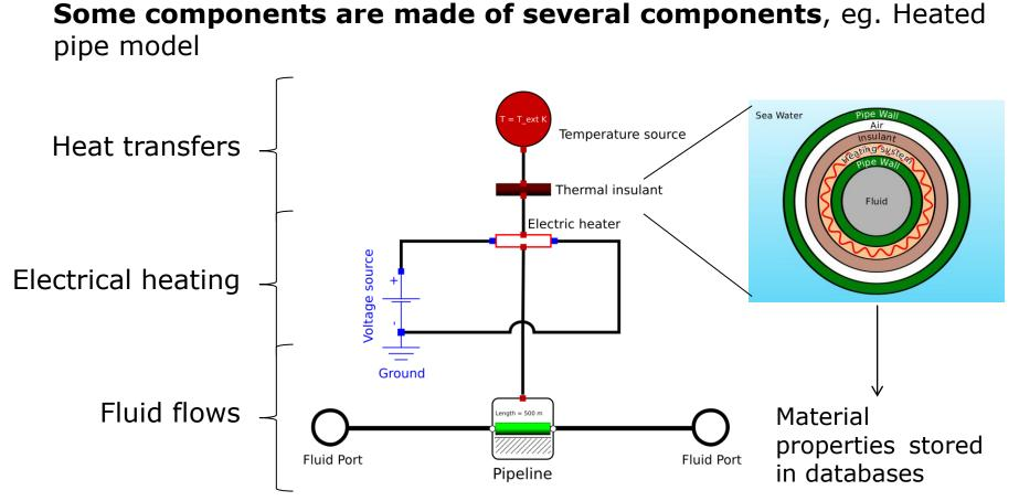
The heated pipe is multi-physics system built in a multi-level approach
