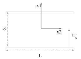
that is, the considered rarefied gas is trapped between two walls of size  $L \times M$  and at distance  $\delta$  from one another, with  $L, M >> \delta$ .
